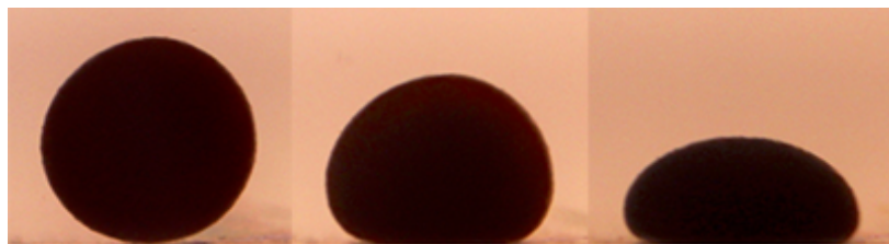
Magnetic flattening of cellular aggregates to measure tissular surface tension (6)
