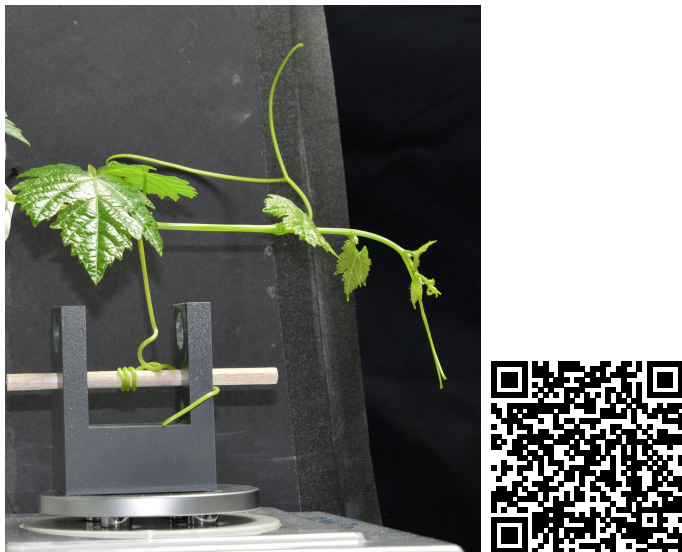
Figure 2: The tendrils pulls vertically, and the force is measured thanks to the scale
